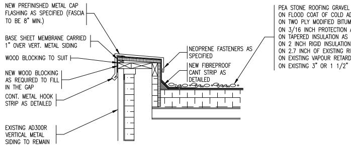
ON FLOOD COAT OF COLD ADHESIVE ON TWO PLY MODIFIED BITUMEN ROOF MEMBRANE ON 3/16 INCH PROTECTION ASPHALT BOARD ON TAPERED INSULATION AS NOTED ON 2 INCH RIGID INSULATION ON 2.7 INCH OF EXISTING RIGID INSULATION ON EXISTING VAPOUR RETARDER
