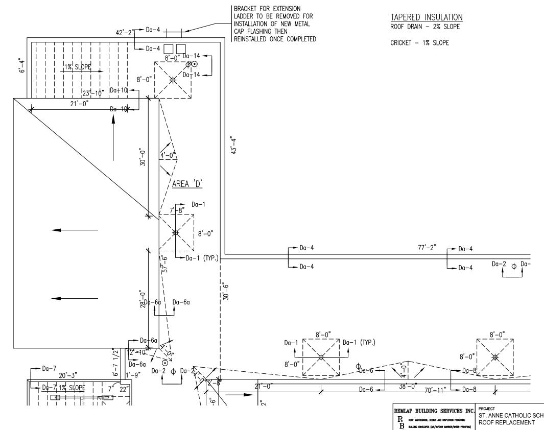
ENLARGED ROOF PLAN - ROOF PENETRATION AND DIMENSIONS
